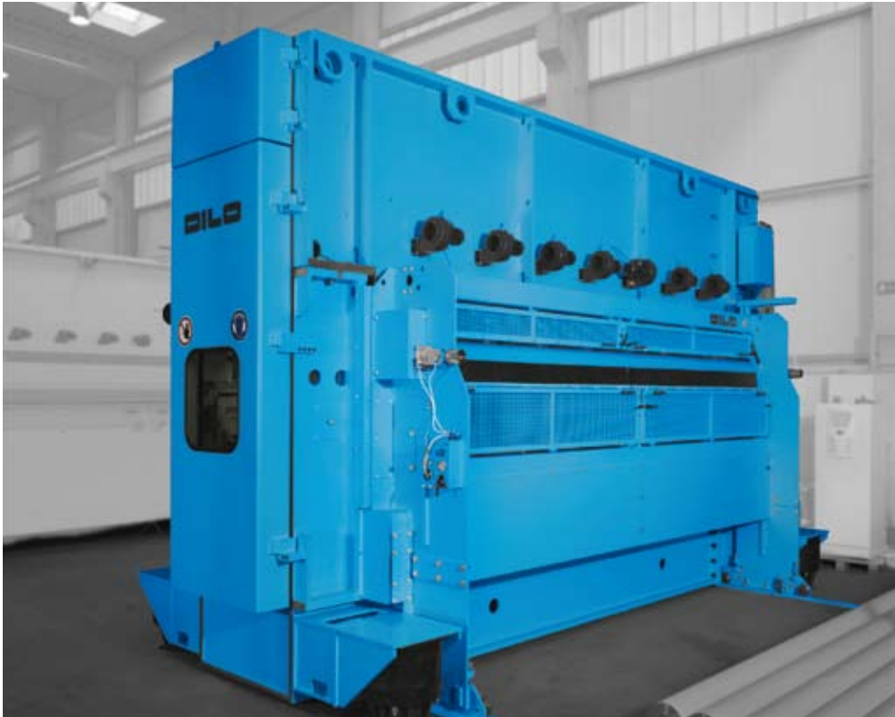
◀ DI-LOOP VSXB 45 working width ww = 4,5 m
