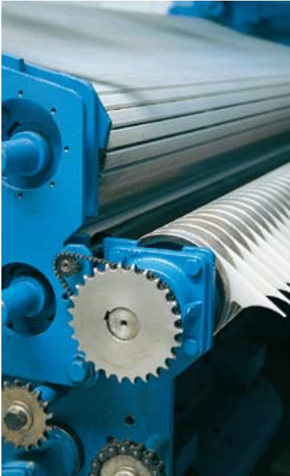
▲ CBF-T System, Transfer roller with finger roller (lower section)
