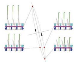
Hyperpunch elliptical needling has been introduced to provide high quality pre-needling and high speed finish needling. The elliptical needling kinematics defines a two-dimensional needle path by a vertical and horizontal stroke motion. The horizontal stroke makes the needle travel with the material while penetrating the fleece.
