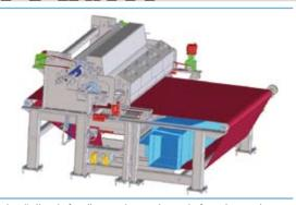
The "Fiberlofter" aerodynamic web forming unit consists of dosing opener, chute feed, feed pan and feed roll, Turbo roll and aerodynamic funnel with suction fan underneath an air permeable screen apron as the web forming section.
