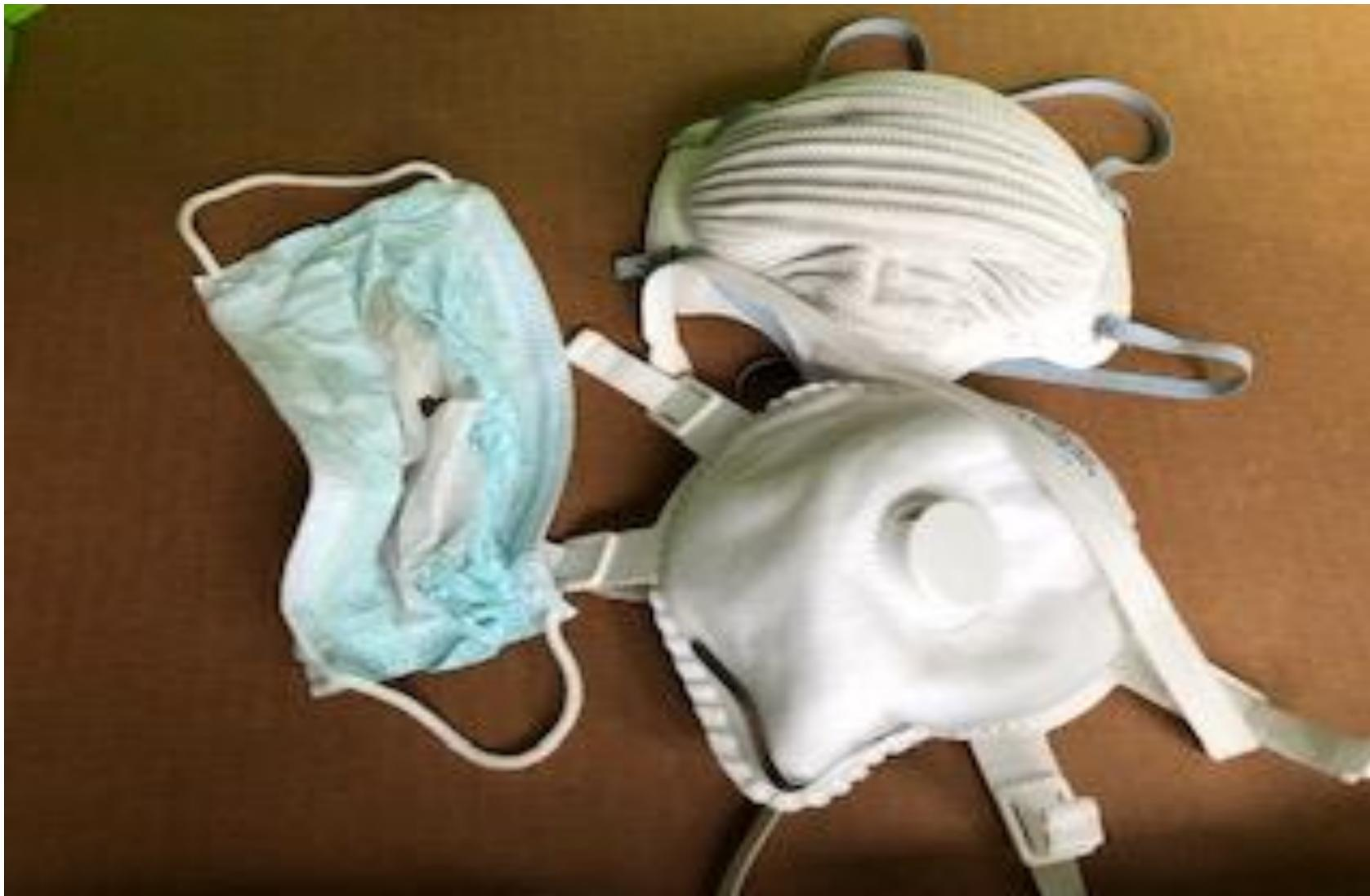
Suspended N95 (L) for ozone treatment for 25 minutes, cracks on rubber band (R).
