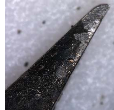
With Oxide Scale
