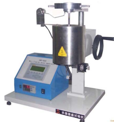
熔指测量仪 Melt Flow Indexer
