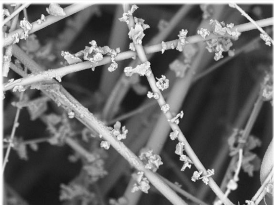
Aerosols captured by the fibers (细纤维捕获颗粒污染物)
