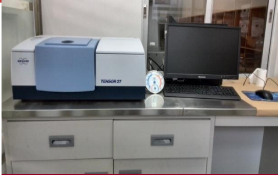
↑ 红外光谱仪 Infrared spectrometer (FT-IR): 测量高分子材料结构 To analysis of polymer structure
