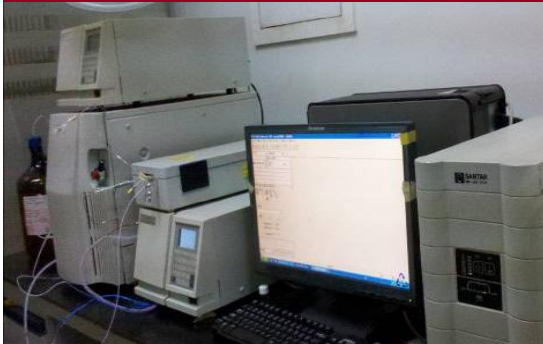
↑ 凝胶渗透色谱仪 GC: 测试树脂分子量和分子分布 To determine MW & distribution in the resin.
