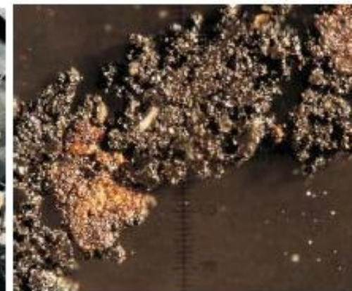
SEM picture: Fouling sample 200 \mu\text{m}
