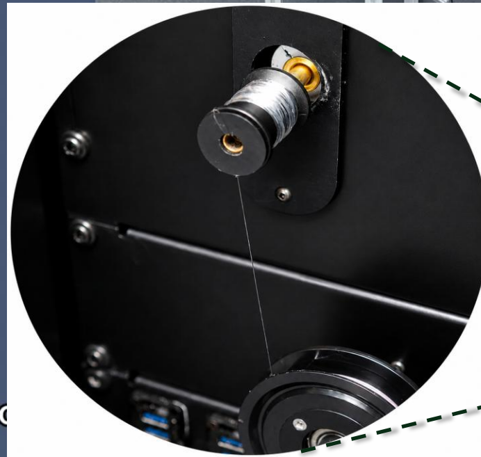
Motorised collecting spool (control fiber speed)
