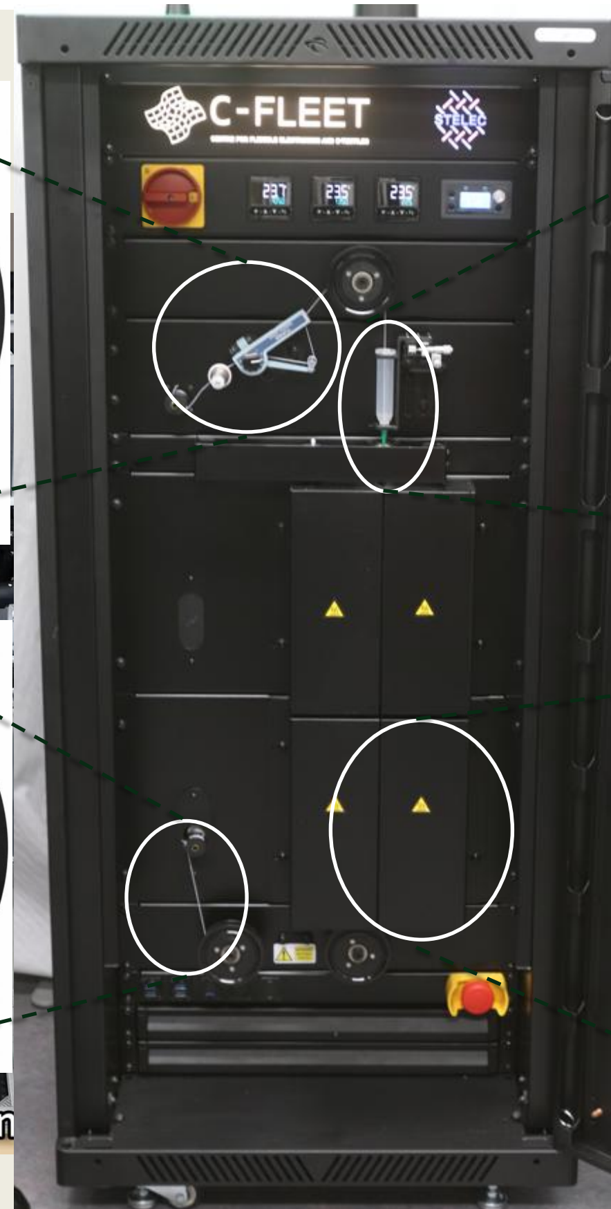
Coating syringe, tapered nozzle, and inspection cameras
