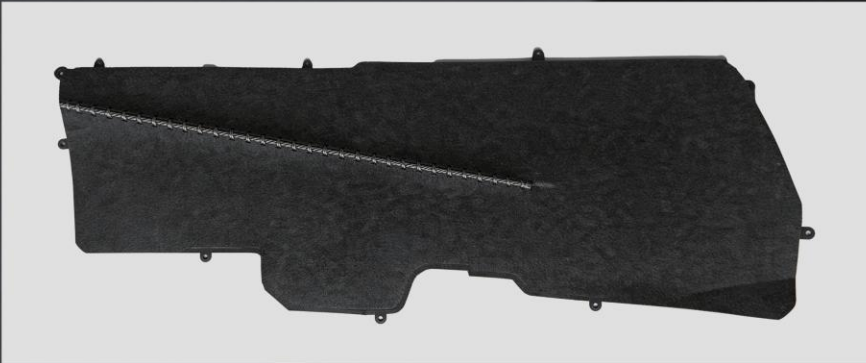
Molded interior panel demonstrator, sewn with recycled PES thread
