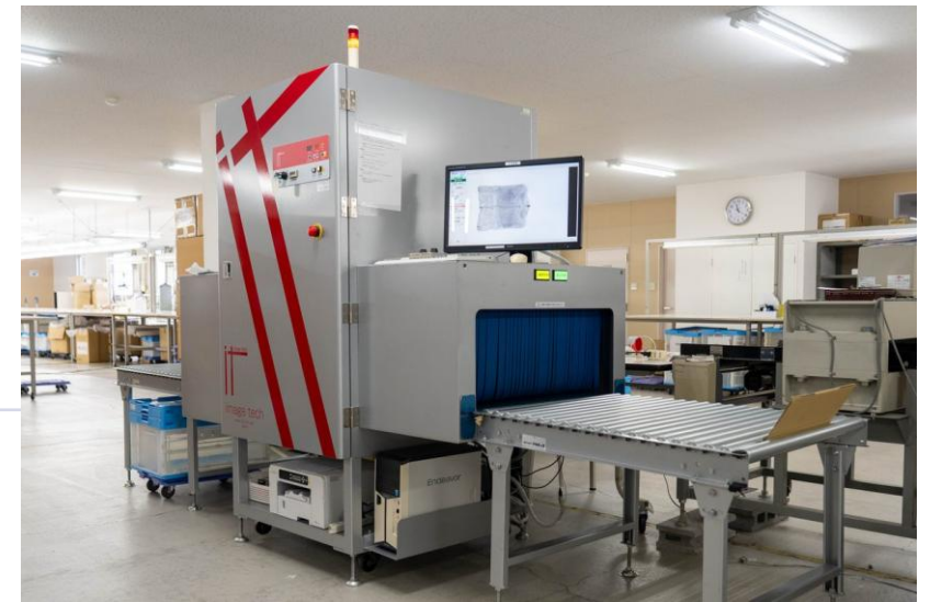
100% verification by X-ray and needle detectors (Hanyu head office)
